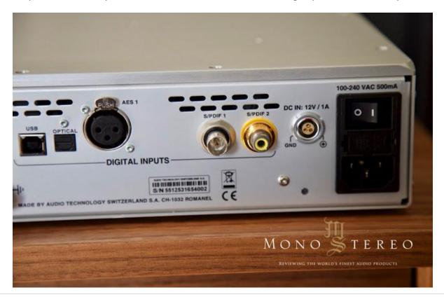
What abut the USB input, that's mostly used? Dedicated high speed USB input was developed around the bit perfect circuit, specially programmed for Nagra by the Italian firm Amanero Technologies.
